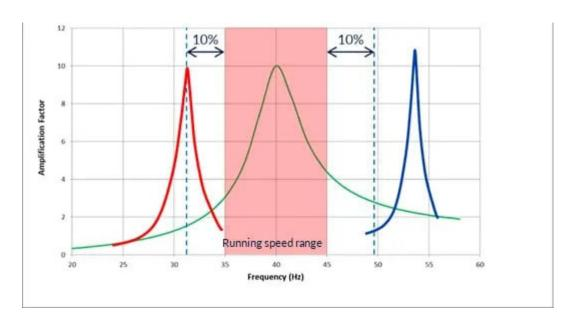
Amplification factor versus frequency showing an example of 10% Separation Margin for variable speed machinery. The green Nf mode is unacceptable as it is within the running speed range. The modes indicated by blue and red meet or exceed a 10% separation margin criteria.
